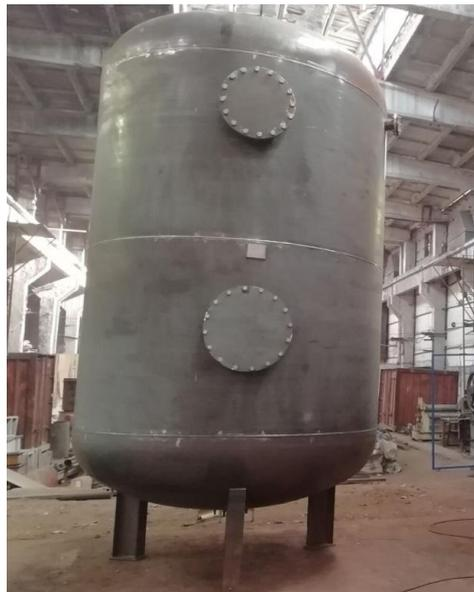
Fig. 1. Example of an industrial mechanical filtration filter. Vertical filtration column
